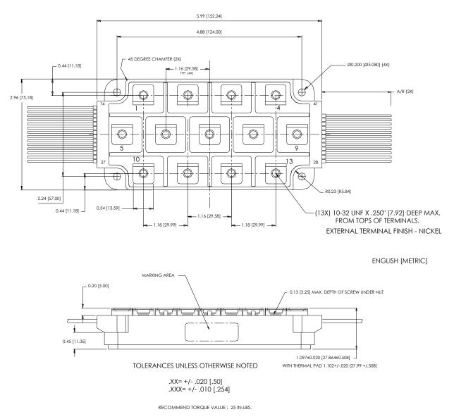
Recommended Thermal Pad Material is Laird Technologies Tgon 805 (to be ordered separately) .
